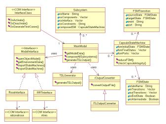
Figure 10: Class Diagram for TDE/UML
