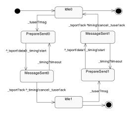
Figure 2: Statechart Diagram for the Transmitter Object
