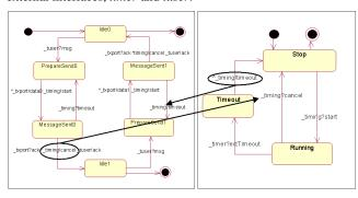
Figure 3: Communicating Transmitter and Timer Components
