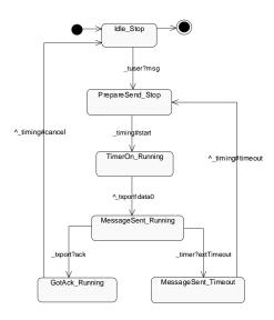
Figure 5: Global Behavioral Model for the *TransmitterTimer*Subsystem
