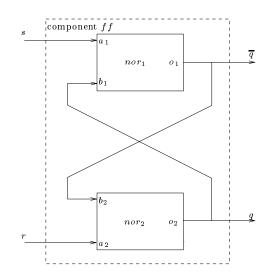
Figure 7.2: RS-flip-flop example
