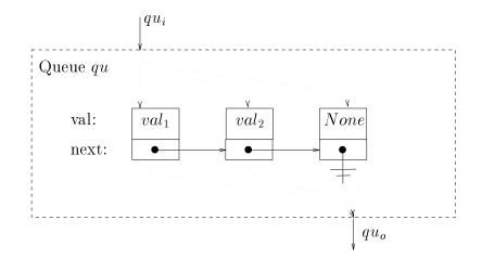
Figure 7.1: Dynamic structure of a queue
