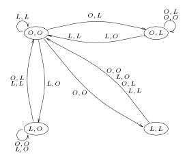
Figure 7.3: Port automaton for the RS-flip-flop
