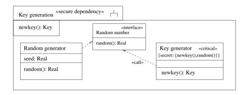
Fig. 4. Key generation subsystem
