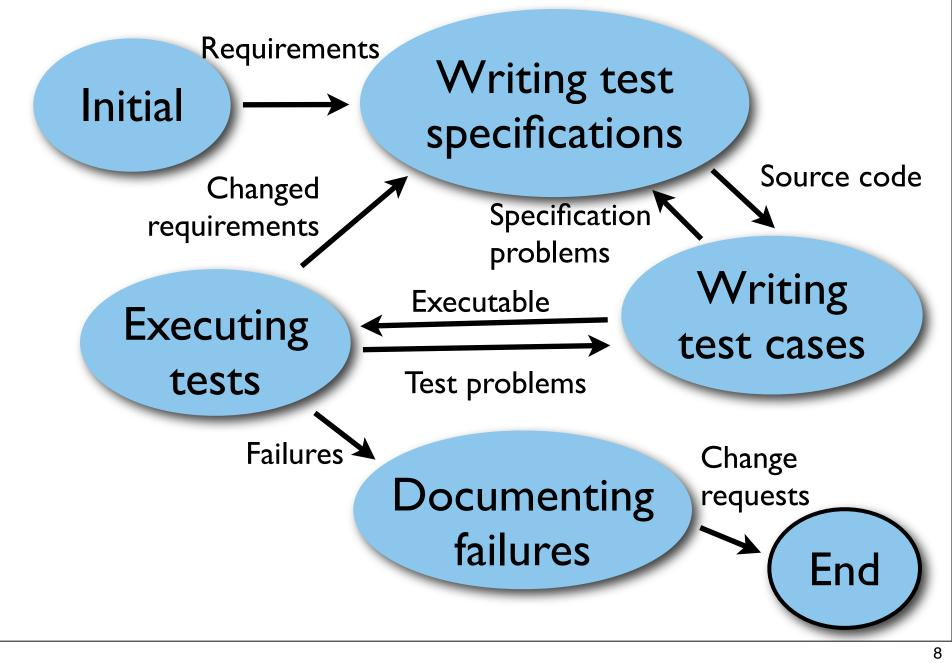
This is an extremely simplified state machine model of a test process. It describes in which states the process can be and what is input and output at state transitions.
