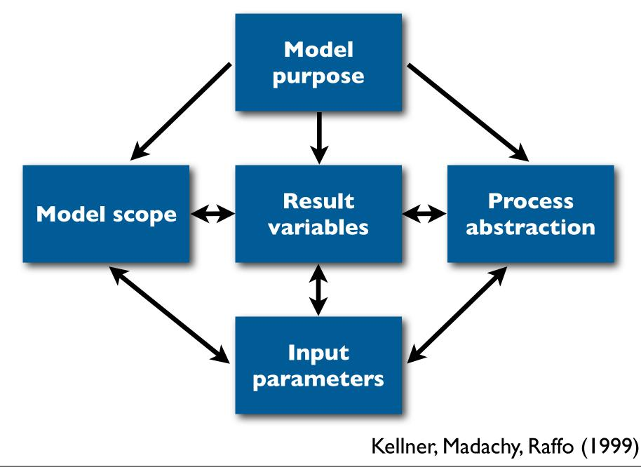
Model purpose: Key questions to address Model scope: Organisational breadth, time span Result variables: Metrics/model outputs designed to address key questions Process abstraction: Level of process detail captured Input parameters: Data and information needed to compute result variables 12
