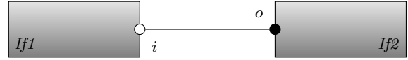
Figure 35 Required connection annotation requiring components of type If1 to be always connected to a component of type If2 through ports i and o , respectively.
