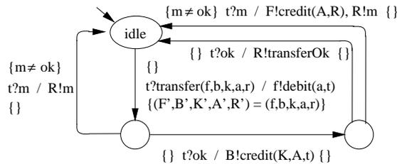
Conceptually, each state transition diagram describes a clerk object with an own state. This object is identified by an identifier variable which will be later bound to the state transition diagram describing the whole object behavior. The state of a clerk object provides the clerk with the data necessary to execute the method.
