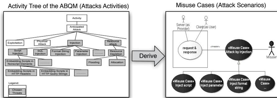
Fig. 4. Using the ABQM for deriving misuse cases
