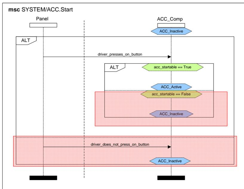
The expressions “driver-presses-on-button”, “driver-doesn’t-press-on-button” are specified by the corresponding events *driver\_presses\_on\_button* and *driver\_does\_not\_press\_on\_button*.
