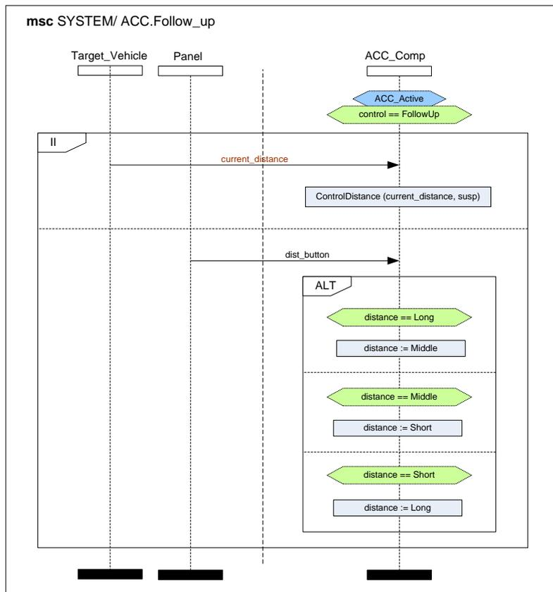
The expression “acc controls following distance to target vehicle” is underspecified in the semiformal specification. Thus, we will underspecify it also on the MSC diagram – we will represent it by the the MSC-block *ControlDistance*. As an input for this block the following distance to target vehicle will be taken – we represent it by the *current\_distance* signal.
