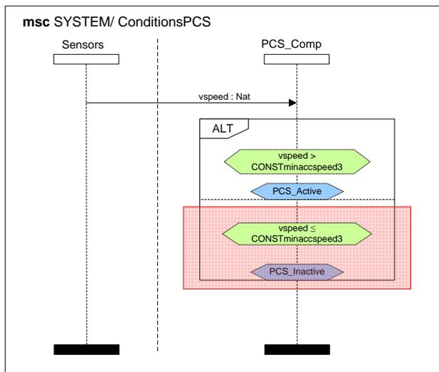
WHILE vehicle speed is lower than  $CONST_{minaccspeed}3\text{km/h}$
